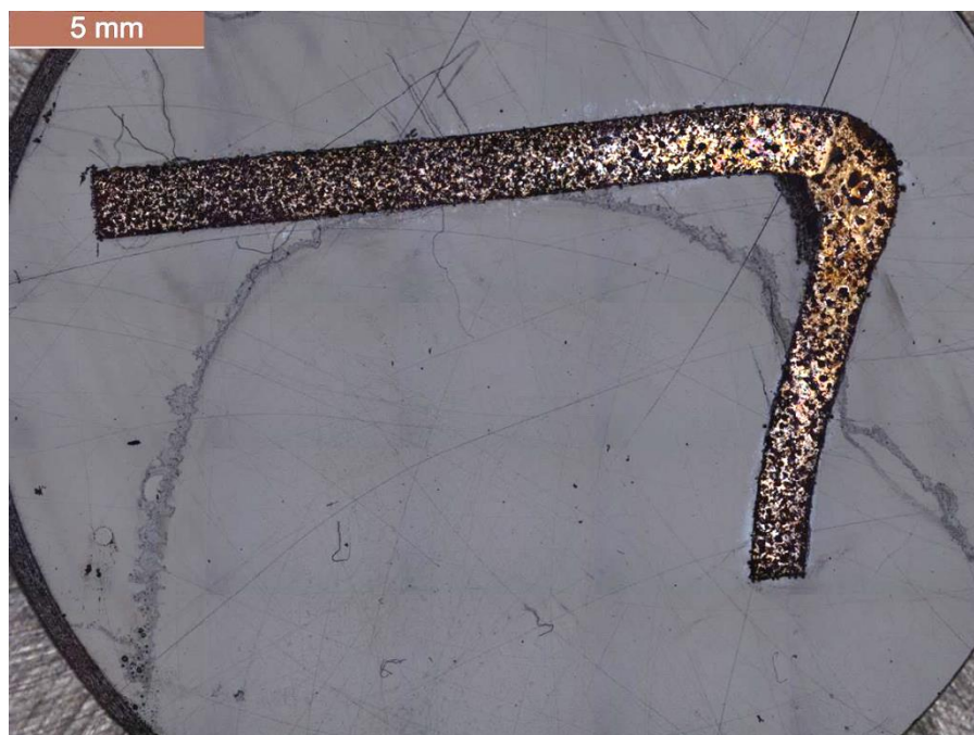
Fig. 4: Optical microscope image of portion of Section "A" of Capsule 2 wall (Image MM2B2-OMS-001).
