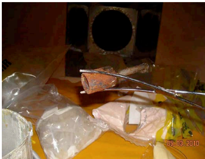
Fig. 1: Photo of a metal tube, presumably containing potentially loose zeolites that had not undergone HIP [18].
